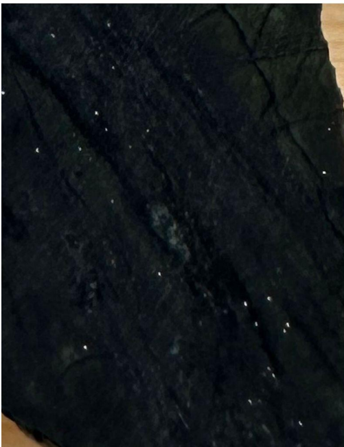
Figure 6: Core sample from drill hole RPM-DDH002 at a depth of 41 meters, showing visible grains of awaruite. The lower images present magnified views of the awaruite grains under a microscope, with sizes up to 428 microns.
