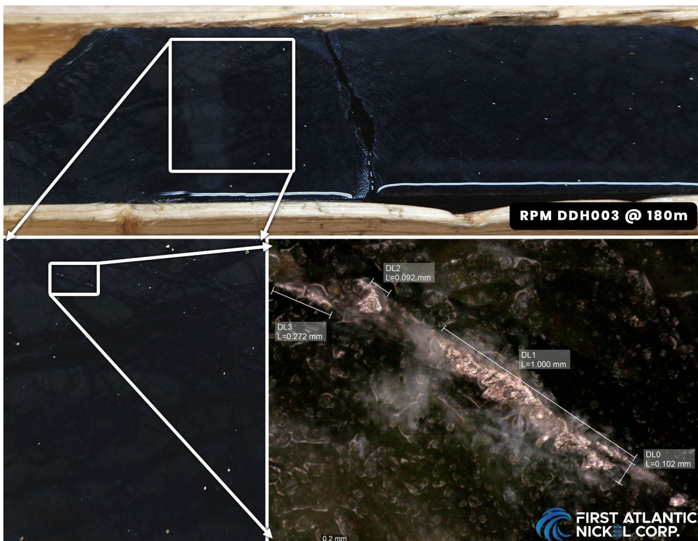
Figure 4: Core sample from drill hole RPM-DDH003 at a depth of 180 meters, featuring visible awaruite. The lower images showcase magnified views of the awaruite grains, displaying smooth and grooved surfaces, with an elongated awaruite nickel-alloy grain up to 1,000 microns in size forming as fracture filling.
