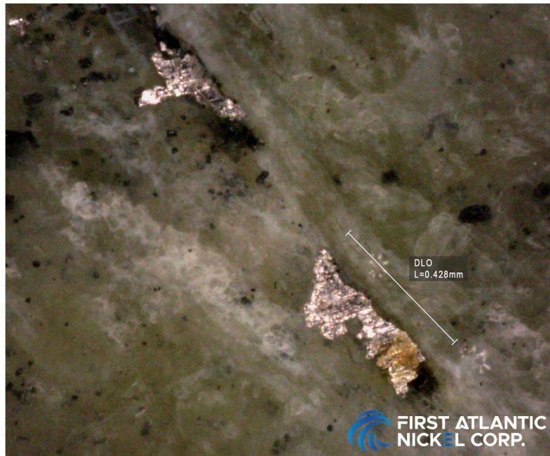
Figure 6: Core sample from drill hole RPM-DDH002 at a depth of 41 meters, showing visible grains of awaruite. The lower images present magnified views of the awaruite grains under a microscope, with sizes up to 428 microns.
